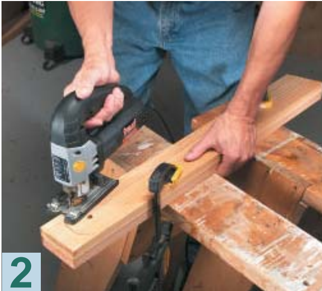
2 CLAMP the leg boards together (rough side in) and cut both of them at once to create identical leg pairs. Drill the 3/8-inch bolt hole in the upper end before unclamping.
