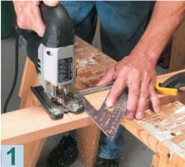
1 CUT THE BOARDS for the top and the frame that supports it using a jigsaw or handsaw and a square. (See the exploded view diagram on next page.)
